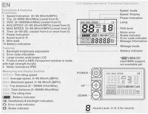
Remark: not all icons are used for the current controller setup. PAS level range is 0-5, no lights are fitted to the Cross5
