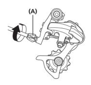
the nature of the used control wire hulls which gets compressed over time. To re-adjust it is usually enough to slightly tighten the gear wires.
