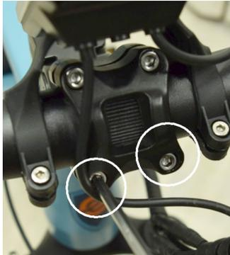
not remove the screw! There are two clamp plates, as soon as both are release you may adjust the angle. Re-tighten properly!
