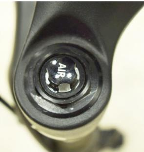
The right side lever allows to adjust the damping of the oil cartridge. If the lever is turned clock wise the damping gets softer – turned to the left it will get harder.
