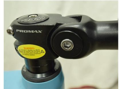
Adjust the tilt of the handlebar by opening two of the handlebar clamp screws (upper or lower, 5mm Allen Key).
